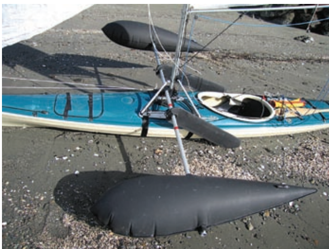
(Top) The Wind Seeker has plenty of sail area to take advantage of light breezes. (Bottom) The sails, spars, outriggers and floats go together as a single self-contained assembly. A pair of straps around the hull and a cord around the cockpit coaming hold it securely to the kayak.
